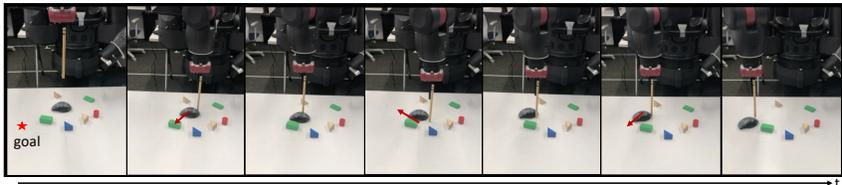
Figure 8: Collision-free pushing on a real-world setup. The task is to push a mouse to a target location without colliding into any obstacles. Our robot can successfully complete the task with 3 push attempts.
